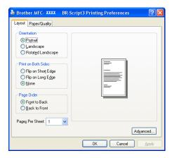
If you are using Windows NT<sup>®</sup> 4.0, Windows<sup>®</sup> 2000 or XP, you can access the **Layout** tab by clicking **Printing Preferences...** in the **General** tab of the **Brother MFC-XXXX** (or **DCP-XXXX**) **BR-Script3 Properties** screen. The **Layout** tab enables you to change various layout settings such as **Orientation**, **Print on Both Sides**, **Page Order** and **Pages Per Sheet**.
